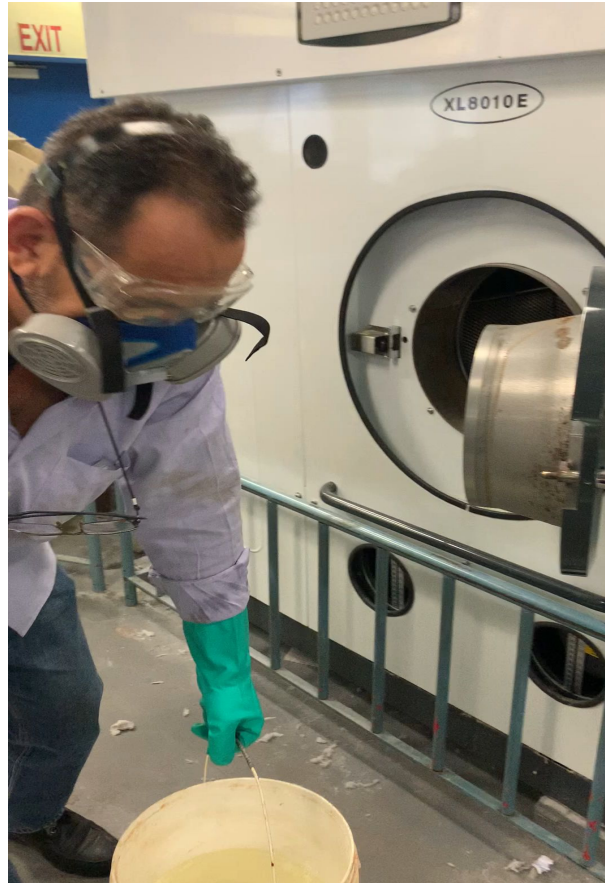
Laundry Maintenance Worker loading Perc into dry cleaning machine (Video)
